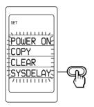
The current interval setting stays lit. The factory setting is 150 ms. (ms: 1/1000 second)
